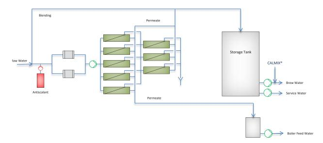
Thus nanofiltration is not ideally suited for the brewing water applications. In special cases, such as the ion exchange plant effluent recycling, nanofiltration can be used successfully. In practical use, the performance of a reverse osmosis membranes can be affected by so-called fouling or scaling. Fouling is organic deposits on the membrane, which are at least partially removed from the membrane surface by suitable cleaning.
