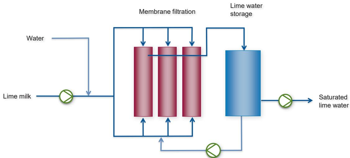
Combined with reverse osmosis and the EUWA LIQUICK® process, saturated lime water from the ELIWA® precipitates the carbonate hardness. After the membrane filtration of the LIQUICK® stage the concentrate thus prepared can be fed again to the reverse osmosis. The combination of reverse osmosis, LIQUICK® and ELIWA® achieves an overall recovery of up to 98 percent.
